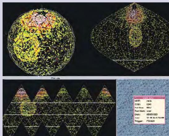
Different projections of the Sudbury Neutrino Detector (SNO) photomultiplier array with two rings clearly present. This event is the result of a high energy neutrino produced from a cosmic ray interaction in the atmosphere on the opposite side of the earth. After passing through the earth, the neutrino interacted in SNO, scattering an electron, which can be seen as the less intense secondary ring. The colour and density are proportional to the energy of the event.
