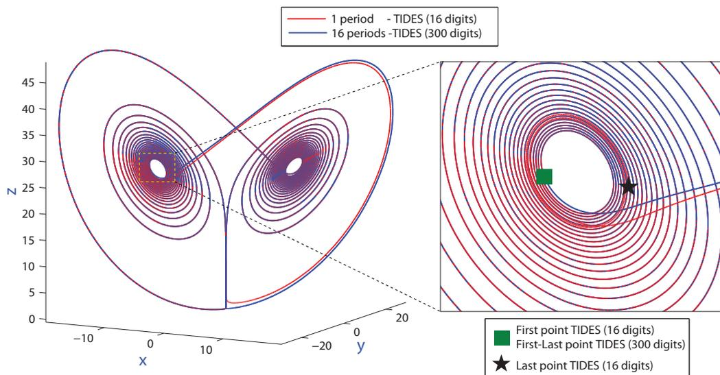
**Figure 3.** Numerical solution of the  $L^{25}R^{25}$  unstable periodic orbit of the Lorenz model for 16 time periods using the TIDES code with 300 digits, compared with just one time period using 64-bit IEEE arithmetic.
