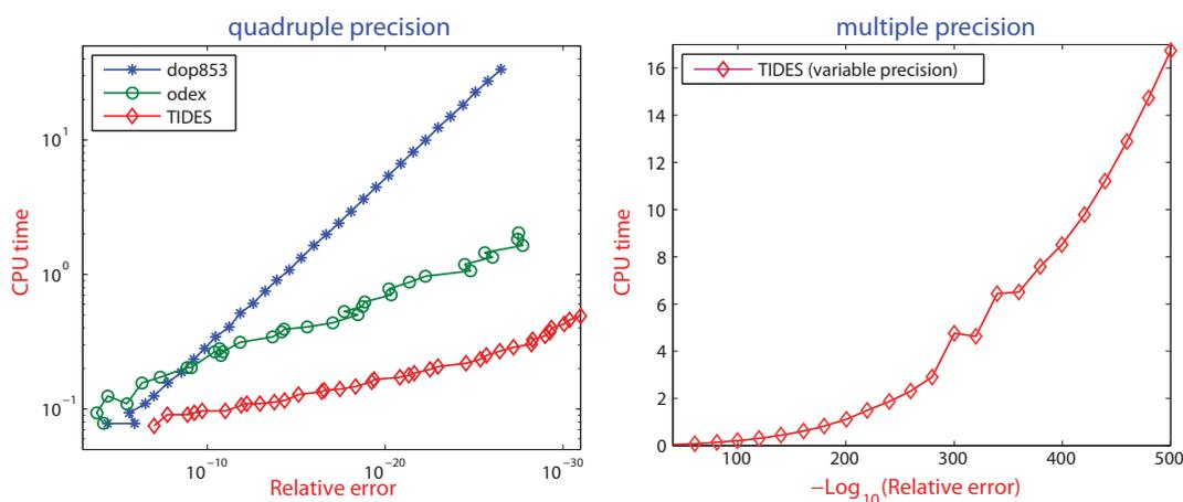
**Figure 2.** Left: Error vs. CPU time for the numerical solution of the unstable periodic orbit LR for the Lorenz model (in double-double arithmetic) using a Runge-Kutta code (dop853), an extrapolation code (odex) [50,51] and a Taylor series method (TIDES). Right: Error vs. CPU time for the numerical solution of an unstable periodic orbit for the Lorenz model (in 500-digit arithmetic) using the TIDES code. Taken from [52].
