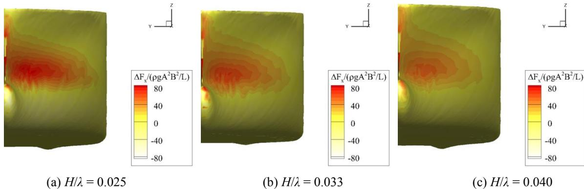
Fig. 5 Added force contours of S-LNGC for different wave slope ( $Fn = 0.188$ , head sea,  $\lambda/L = 1.0$ )
