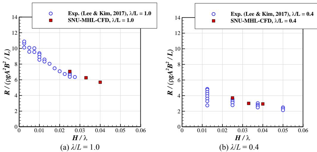
Fig. 4 Added resistance of S-LNGC for different wave slope ( $Fn = 0.188$ , head sea)
