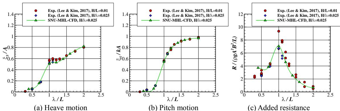
Fig. 3 Motion responses and added resistance of S-LNGC ( $F_n = 0.188$ , head sea)
