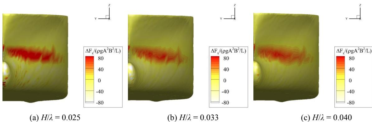
Fig. 6 Added force contours of S-LNGC for different wave slope ( $Fn = 0.188$ , head sea,  $\lambda/L = 0.4$ )
