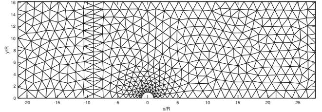
Figure 2: Illustration of mesh. Free surface plane including a wave generation zone.
