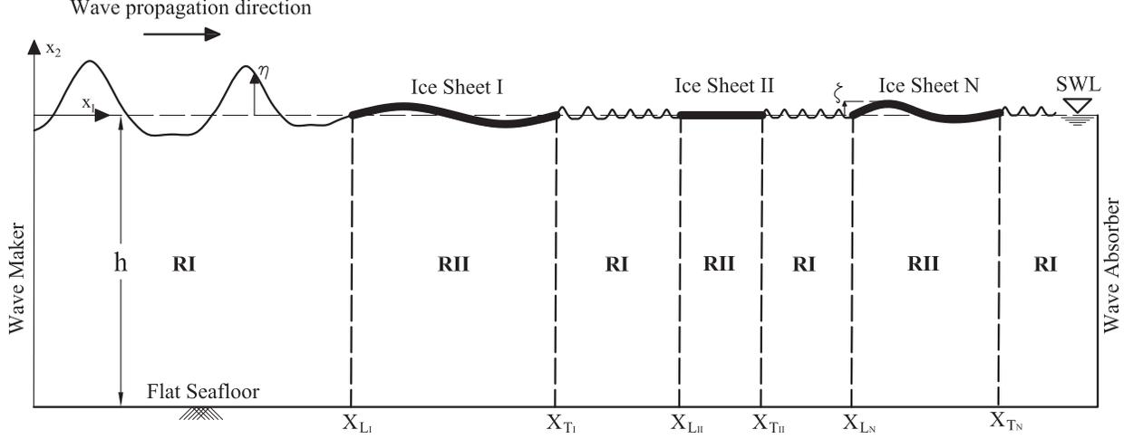
Figure 1: Schematic of the theoretical wave tank of two-dimensional wave interaction with floating, deformable ice sheets. Only three ice sheets are shown here, and these may be  $N$  in general. Also shown, are the two types of regions discussed within the text. Figure not to scale.
