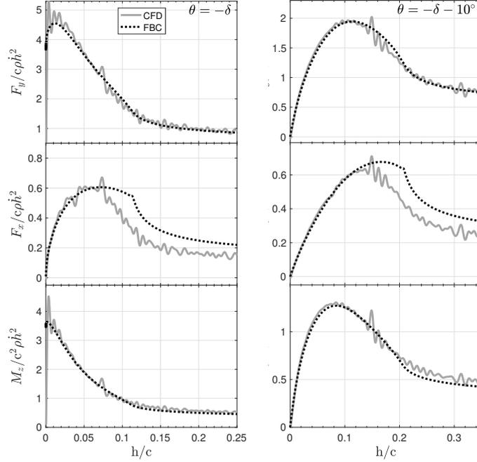
Figure 3: Same as Fig. 2 for two other inclination angles:  $\theta = -\delta$  (left) and  $\theta = -\delta - 10^\circ$  (right).  $\delta \simeq 18.1^\circ$  is the half opening angle of the foil trailing edge. For  $\theta = -\delta$  the trailing edge contour is tangent to the initial free surface.
